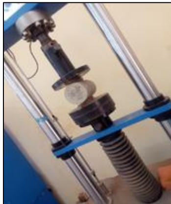
Figure 3 Splitting tensile test on cylindrical concrete specimen (100 mm × 200 mm)
