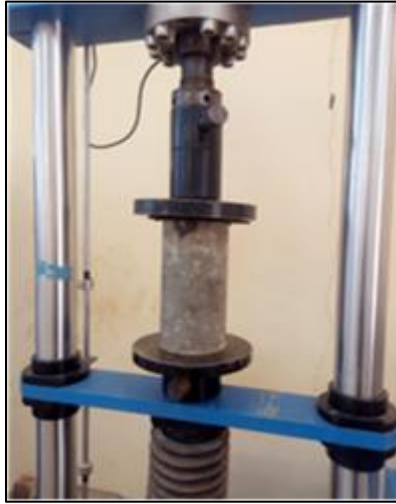
Figure 2 Illustration of the compressive strength test performed on a 100 × 200 mm concrete specimen
