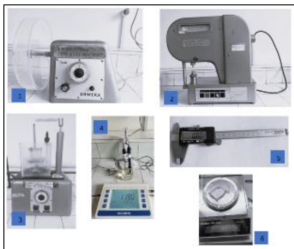
(1: Friability tester; 2: Hardness tester; 3: Disintegration tester; 4: pH-meter; 5: Digital caliper; 5: Precision scale)
