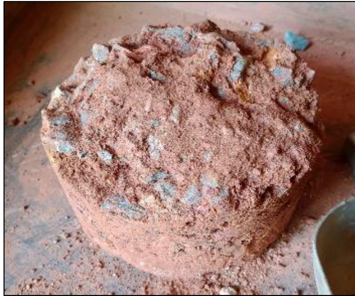
Figure 15 Sample after compaction containing crushed gravel
