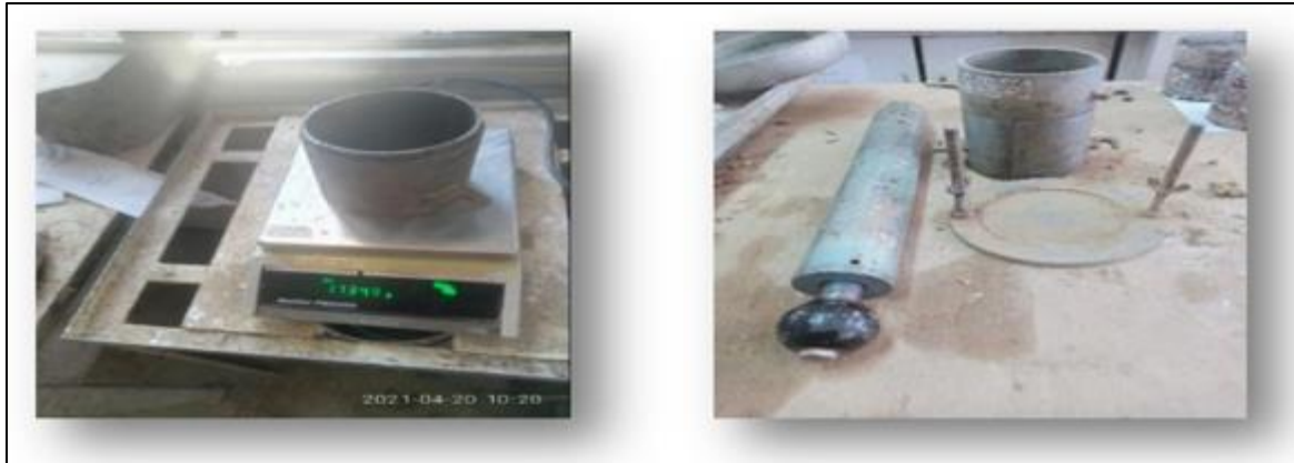
Figure 11 Proctor test equipment [14]
