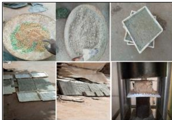
Figure 14 Production of paving stones made using the new material and practical test of compressive strength in the laboratory
