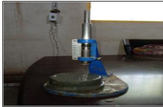
Figure 8 Cement test (Vicat apparatus equipped with a needle and an overload)
