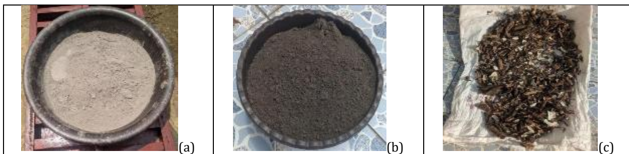
Figure 1 Materials used in the preparation of cement paste cubes. (a) Cement; (b) Cassava peeling Ash; (c) Cassava peels
