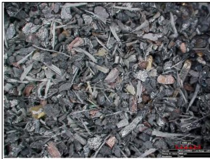
Figure 3 Digital optical microscope image of the fraction of magnetic particles containing non-magnetic metals
