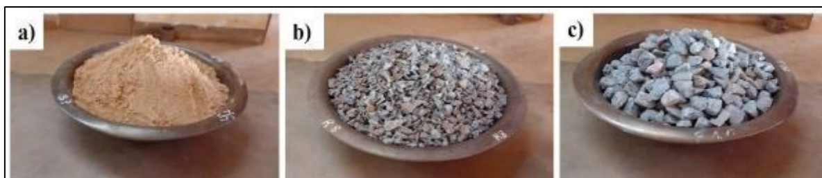
Figure 1 Aggregates used for the study: sand (a), 5/15 gravel (b), and 15/25 gravel (c)
