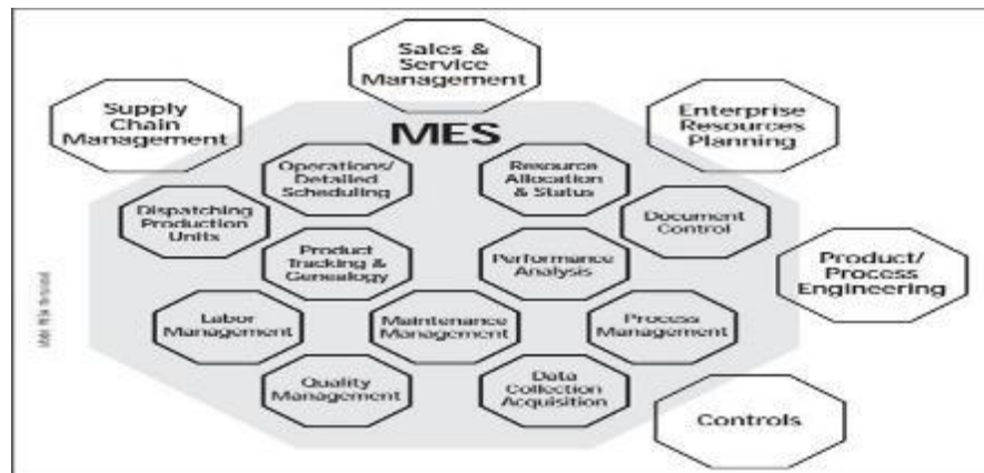
Figure 2 Illustration of MES functions and their interconnections with other systems. The extent of these linkages can vary depending on the specific application. Source: [9]
