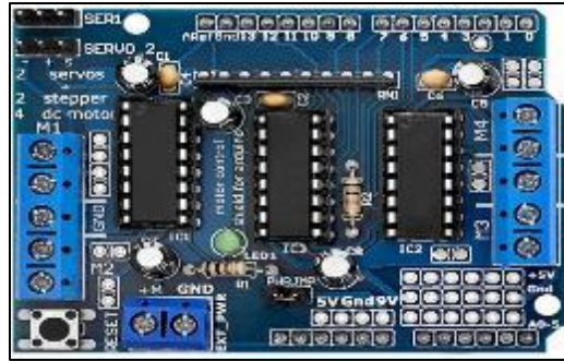
Figure 2 L293D Motor Driver (adapted from Az-Delivery, 2025)
