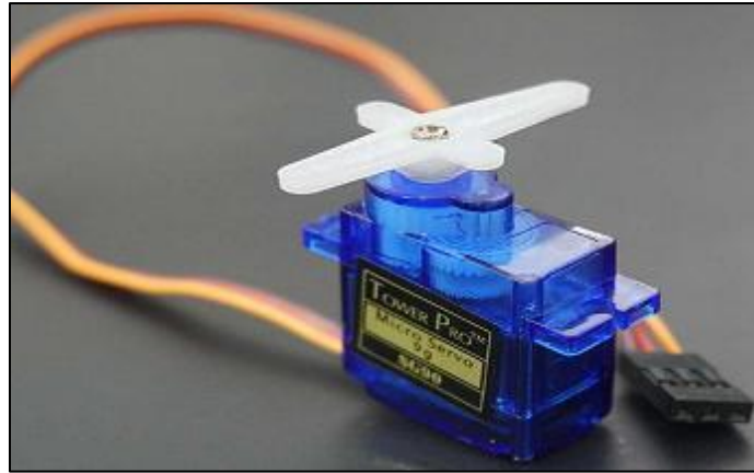
Figure 8 Sg90 Servo Motor (adapted from ElectronicsWings, 2025)
