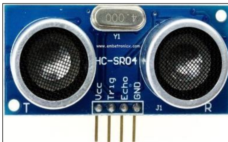
Figure 5 HC-SR04 Ultrasonic Sensor (adapted from Embe Tronicx, 2025)
