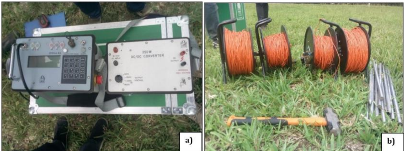
Figure 3 Electrical resistivity measurement equipment: a) a Syscal R2 and an electrical current amplifier, and b) four electrical cable coils, a hammer, and electrodes
