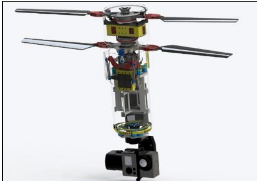
Figure 1 Dual-Engine Variable-Pitch Multirotor UAV
