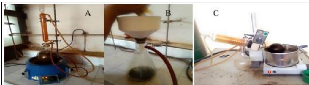
Figure 2 Plant extraction process: A: Decoction; B: Filtration; C: Evaporation
