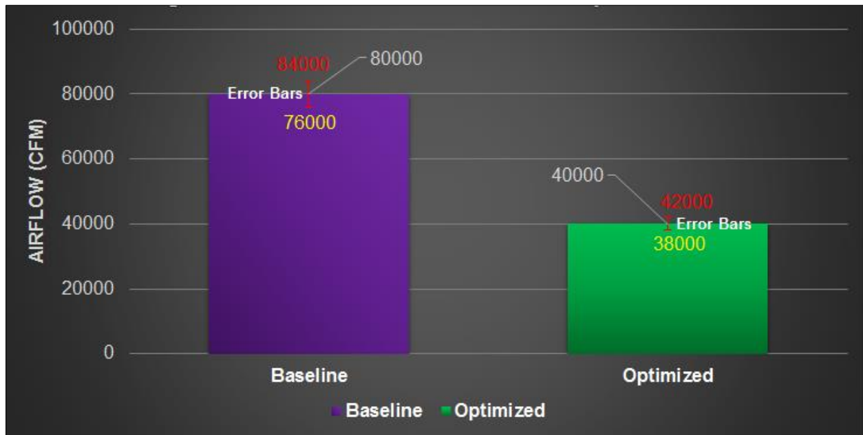
Figure 2 a Airflow reduction from 80,000 CFM to 40,000 CFM (50% improvement) after optimization, maintaining 9,500 particles/ft 3 (ISO 7), with \pm 4\% error (95% CI: \pm 3.2\% , p < 0.001 ) from 150 simulations
