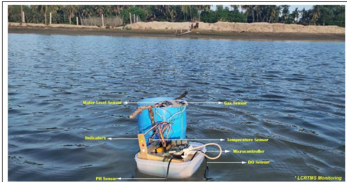
Figure 2 IoT Water Quality Prototype. Source; (Sivakumar and Ramya, 2021)
