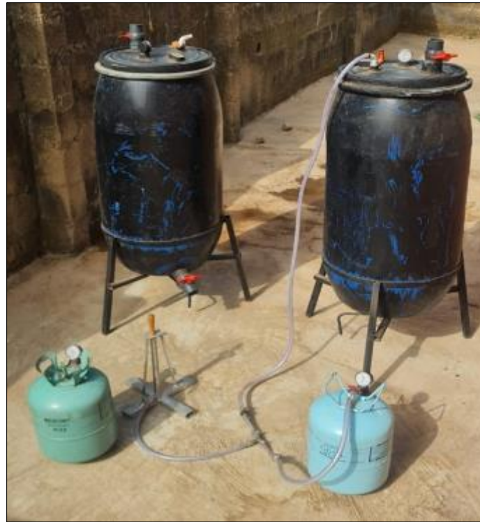
Figure 15 Experimental Setup for Biogas Production by Co-digestion Process
