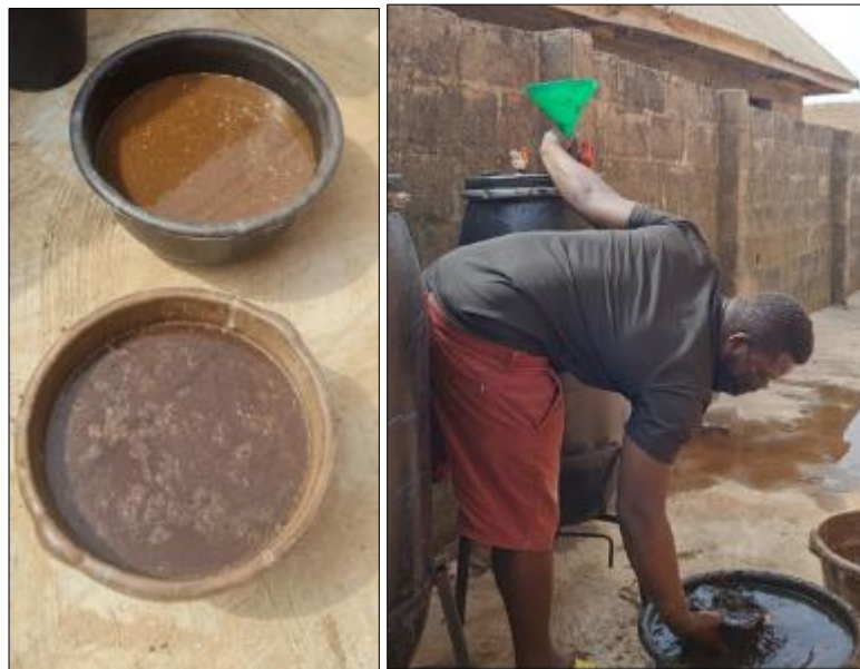
Figure 14 (b) Prepared Slurry Figure 14 (c) Loading of Digester
